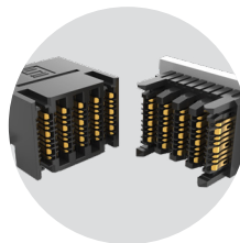
In Development: 2 Pair Design for a Lower Profile
