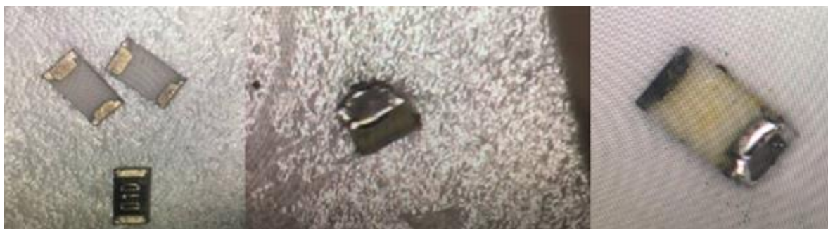
Fig. 2 Examples of poor solderability, poor wetting, and moisture damaged terminations
