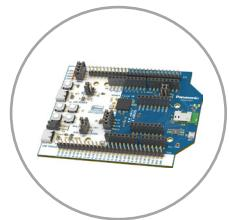
Easily access all the different module interfaces like USB, UART, NFC, and GPIOs, which makes the evaluation board ideal for the evaluation of the module as well as rapid prototyping of products. All GPIOs are led out via pin headers, and the Arduino form factor allows the connection of shields available on the mass market.
