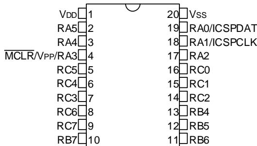
**Figure 2-3.****20-Pin VQFN**
