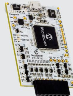
The MPLAB Snap programs quickly. It features a powerful 32-bit 300 MHz SAM E70 Arm® Cortex®-M7 based MCU for quicker debug iterations. Along with its support for a wide target voltage, the MPLAB Snap supports advanced interfaces such as 4-wire JTAG and Serial Wire Debug with streaming data gateway. It is also backward compatible for demo boards, headers and target systems using 2-wire JTAG and In-Circuit Serial Programming™.
