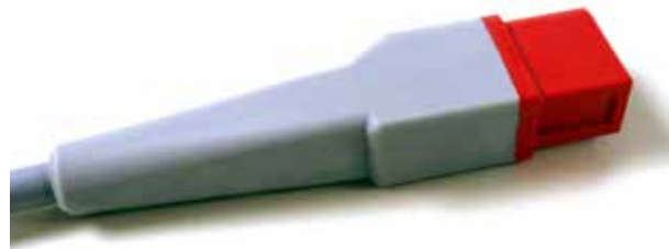
Smooth Strain Relief: A smooth, solid strain relief is typically less flexible but is easier to clean as compared to a segmented strain relief
