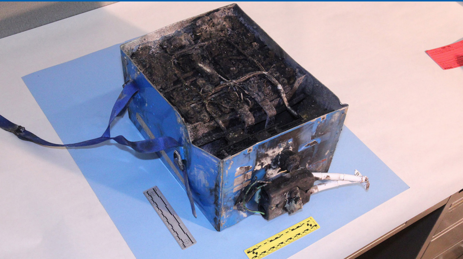
Figure 1: By the time a situation has reached catastrophic thermal runaway, it is too late to manage heat. (Orange County Sheriff's Department/National Transportation Safety Board via AP)
