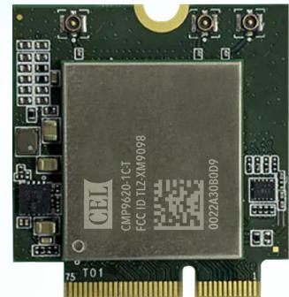
NEW WIRELESS DEPLOYMENTS DEMAND MORE DATA THROUGHPUT AND MORE EFFICIENT NETWORK UTILIZATION. CEL DESIGNED THE CMP9620 TO DELIVER BOTH WHILE OFFERING OUT-OF-THE-BOX INTEGRATION INTO NXP'S I.MX8 ECOSYSTEM. SIMULTANEOUS DUAL-BAND OPERATION, COMBINED WITH CONCURRENT BLUETOOTH AND THE LATEST BLUETOOTH FEATURES, DELIVER THE CONNECTIVITY DEMANDED BY EDGE GATEWAYS AND HIGH-BANDWIDTH APPLICATIONS
