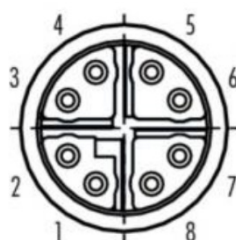
Figure 1 – M12 Connector PIN Layout
