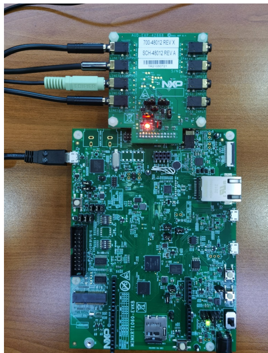
Figure 2. Connection between RT1060 EVKB and audio card
