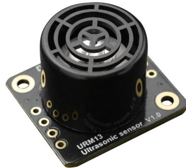
The URM13 Ultrasonic Sensor features excellent sensitivity, automatic noise detection, real-time calibration, HC-SR04 compatible, 1cm resolution, and 1% accuracy.
