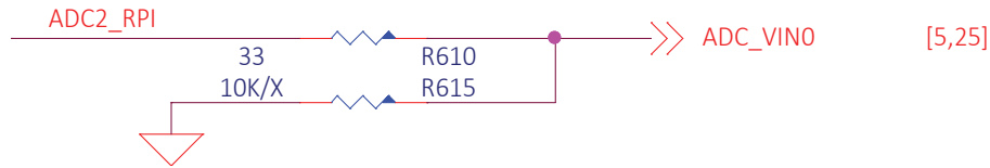
Figure 73: ADC reference circuitry
