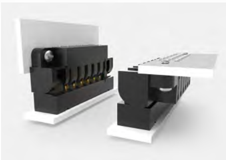
"Hinging" for 90° mating radius, ideal for blind mating (FMPT/FMPS)
