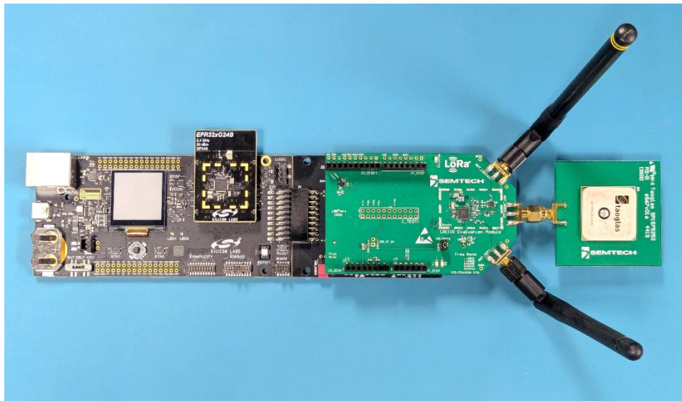
Figure 1, Assembled EFR32 + LR1110 (passive) kit
