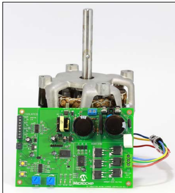
FIGURE 1: AC INDUCTION MOTOR WITH THREE-PHASE INVERTER BOARD
