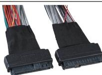
PCI (Peripheral Component Interconnect) Express is a point-to-point connection, which does not share bandwidth but communicates directly with devices via a switch that directs data flow. It also allows for hot swapping or hot plugging and consumes less power than PCI. SFF-8639 is designed for enterprise class backplane interfaces and meets the 12 Gbps electrical performance requirements as defined by SAS-3.0.
