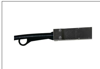
I/O solutions supporting Ethernet and Fibre Channel applications. QSFP+ copper assemblies provide a high density, high bandwidth solution at low cost and reduced power budget. Amphenol's high speed cable assemblies meet and exceed industry standards for performance and reliability as per SFF-8436 & IEEE 802.3ba.
