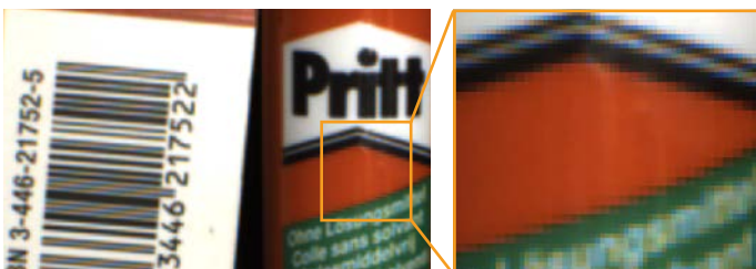
With standard 2×2 debayering, artefacts such as saw-tooth distortion or zip effects compromise the image quality considerably.
