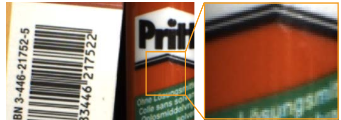
PGI 5×5 debayering clearly improves the edges in the image.
