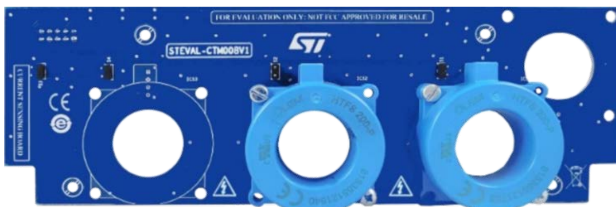
Figure 8. STEVAL-CTM008V1 current sensing board
