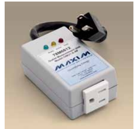
Figure 2. A ZigBee®-based outlet-monitoring unit.
