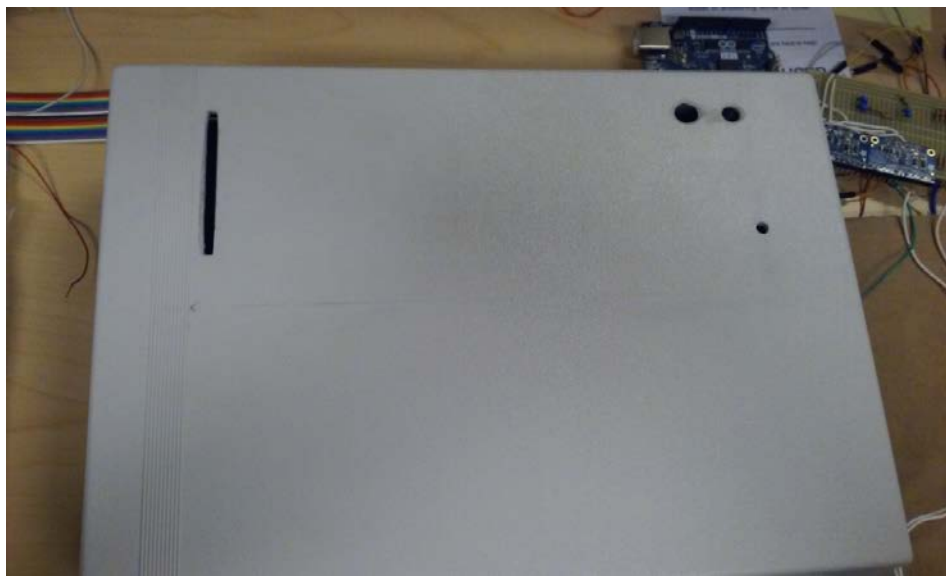
5 Enclosure lid with peripherals' holes drilled.
