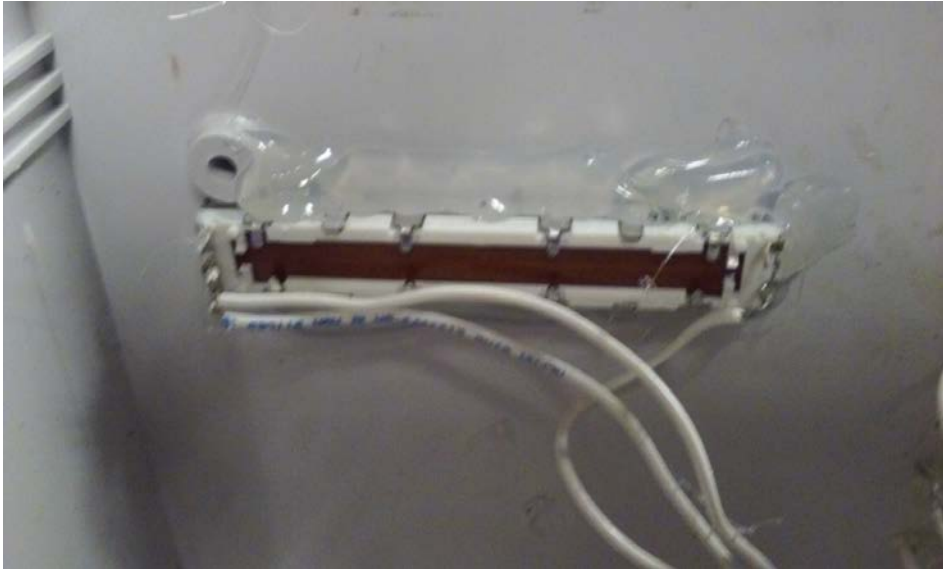
8 Volume Slider glued and wired up.
