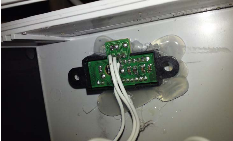
9 IR sensor glued and wired
