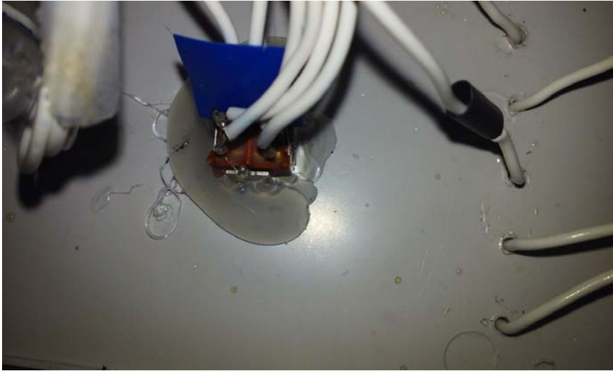
7 Mode switch wired and glued.
