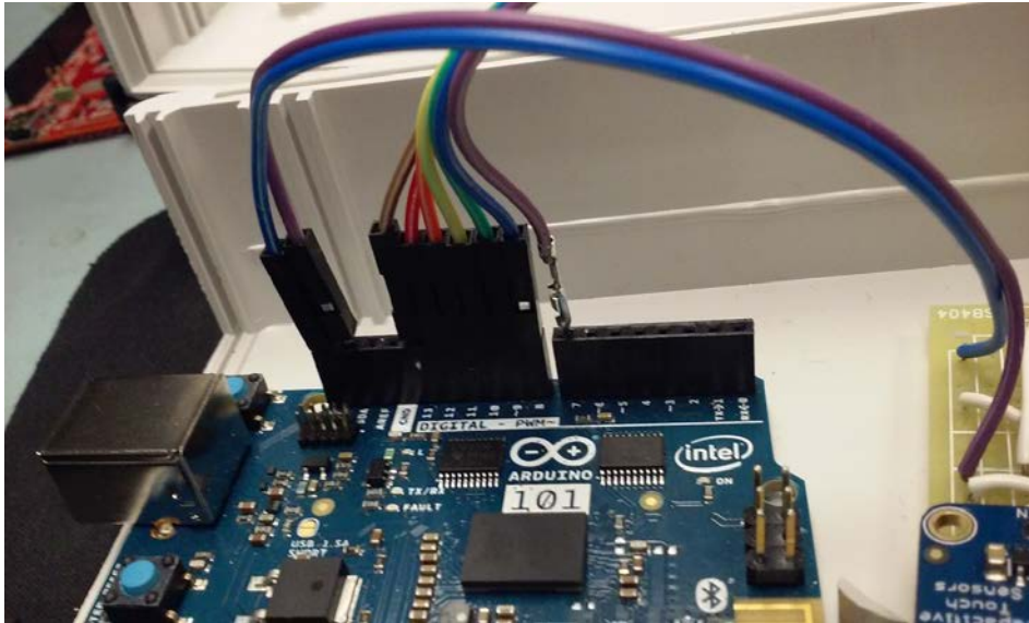
15 Digital Pin outs (7-13) and I2C jumpers (SDA in purple, SCL in blue)
